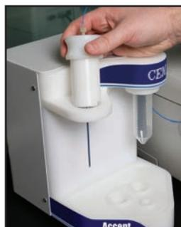
15. Turn on the Accent. Remove the luer cap and insert the vessel into the Accent baseplate to drain the cleavage mix containing the peptide into the centrifuge tube.
