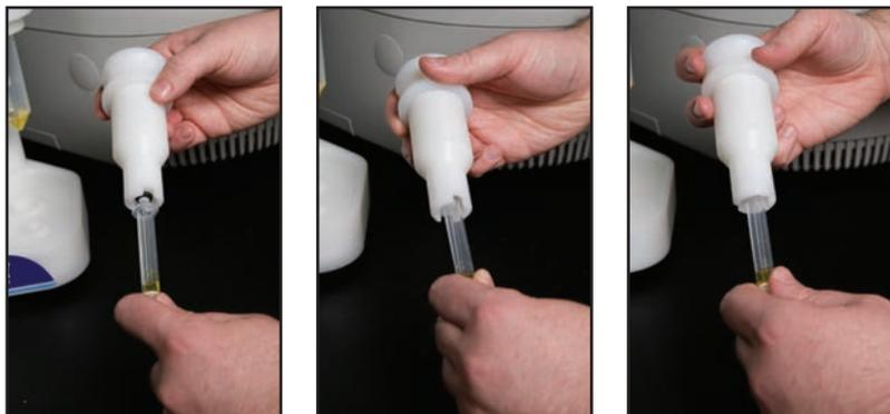
2. Place a yellow ferrule onto the thermowell so that the thinner side of the ferrule points towards the open end of the thermowell.
