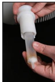
10. Insert the fiber optic probe into the thermowell. Ensure that the thermowell reaches the bottom of the vessel and that the fiber-optic probe is completely inserted into the thermowell.
