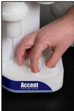
2. Insert a new, clean reaction vessel into the baseplate.
