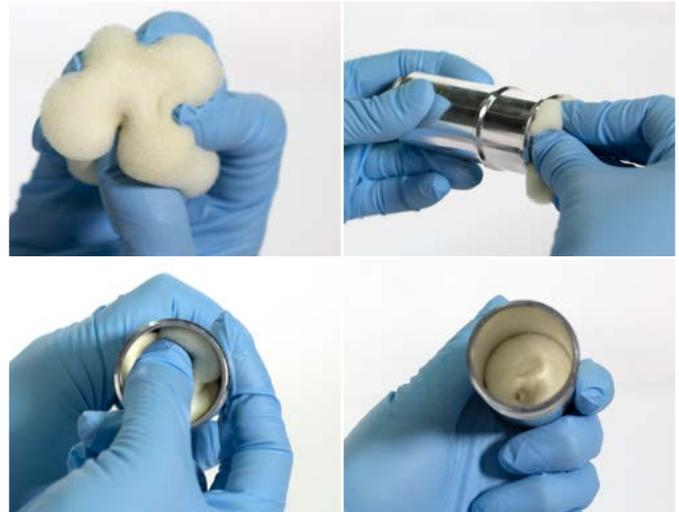
**Image 1:** Insertion of large PUF filter into a Q-Cup
