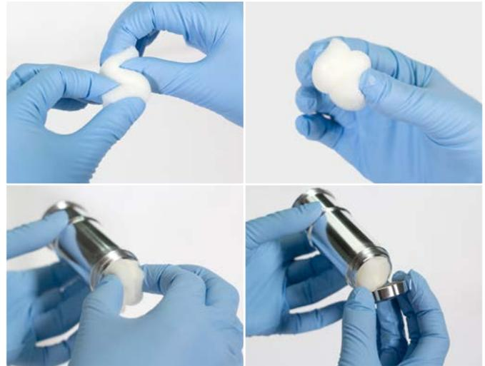
**Image 2:** Insertion of small PUF filter into a Q-Cup
