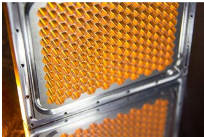
Figure 2. Multiple technological advancements are built into the SMART 6. Its honeycomb lattice, for example, provides collimated infrared radiation for sample heating, therefore avoiding stray light. This allows for highly accurate temperature control.
