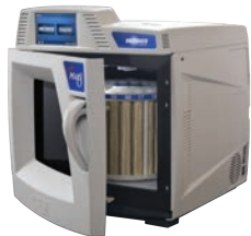
Figure 1. MARS 6 with 75 mL MARSXpress Vessels
