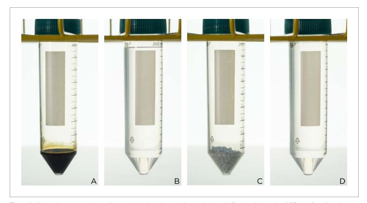
**Figure 4**. All samples were completey digested producing clear, colorless solutions. (A) Bunker oil (max size 0.25 g) before digestion. (B) Bunker oil after digestion (sample diluted to 50 mL), showing clear results. (C) PET (pellet max size 0.25 g) before digestion. (D) PET after digestion (sample diluted to 50 mL), showing clear results.
