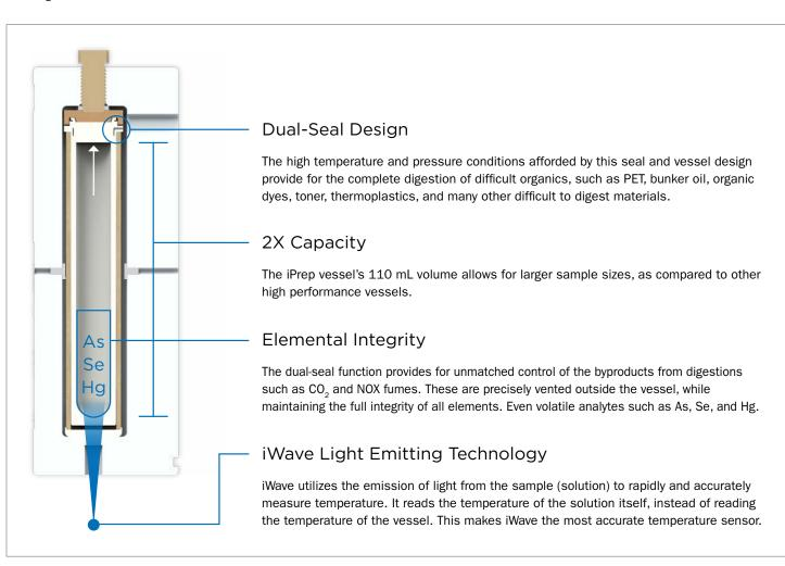
Figure 1. iPrep Vessel Diagram
