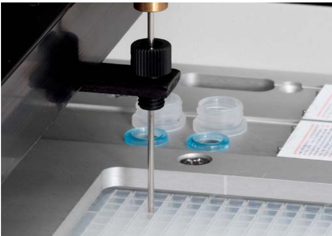
Dissolved peptide-cellulose conjugates in 384 well plate being spotted onto CelluSpots slides.
