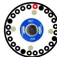
● = Empty Position    ● = Standard Vessel    ● = Control Vessel    ● = Peg
