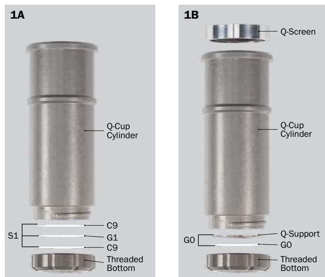
**Figure 1.** Positioning of the G1 and C9 Q-Discs, used in the extraction of the non-hydrolyzed samples (A) and the positioning of the Q-Support and G0 Q-Disc, a combination called G0 used in the extraction of the hydrolyzed samples (B).
