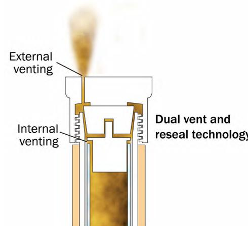
Figure 5. External venting of glass insert
