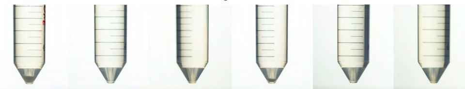
Figure 6. Clear particulate free digested samples
