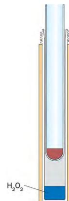
Figure 2. Vessel with hydrogen peroxide and disposable glass insert
