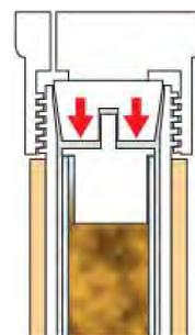
Figure 4. External pressurization of glass insert
