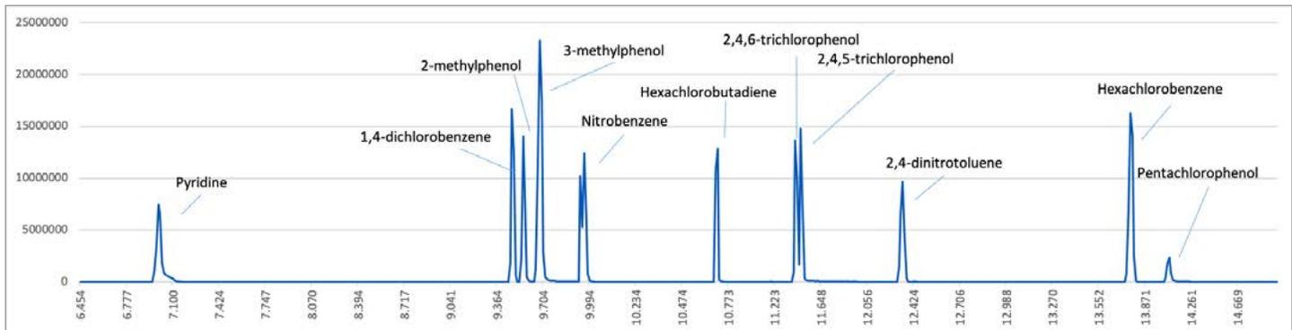
**Figure 1.** GCMS Chromatogram of the SVOCs Extracted from Clay
